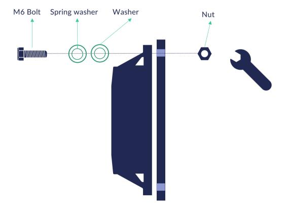
1. Use the appropriate size of screws, it is recommended to use the M6 type and to use Loctite glue on the screws.
