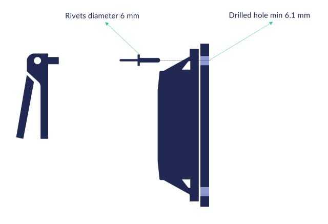
Use the appropriate size of rivets, we recommended to use rivets with a diameter of 6mm.
