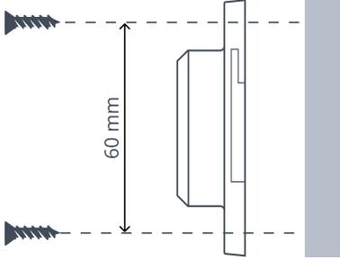
The spacing between the mounting holes when affixing the tag using rivets, screws, or bolts.
