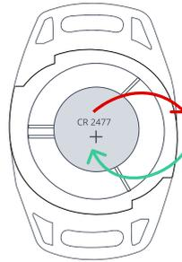
Replace the empty CR 2477 battery with a new one.
