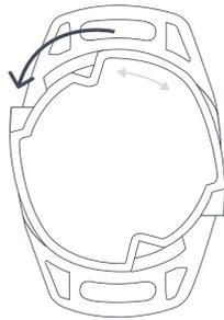
Unscrew the backplate by turning it counterclockwise
