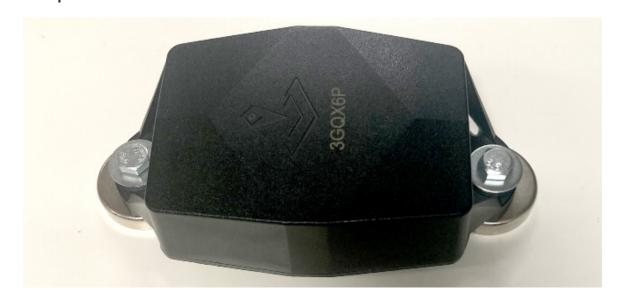
Tighten the screws on the magnets.
