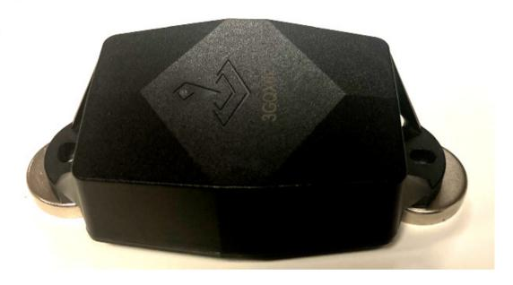
Place the tracker on the magnets. Make sure the metal protection on the magnets is facing up.
