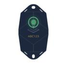
Green LED is **blinking** for minimum 30 seconds.
