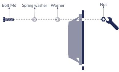
1. Use the appropriate size of screws, it is recommended to use the M6 type and to use thread locking glue on the bolts. We recommend Loctite Thread Locker Blue 242.
