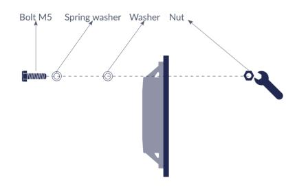
1. Use the appropriate size of screws, it is recommended to use the M5 type and to use thread locking glue on the bolts. We recommend Loctite Thread Locker Blue 242.
